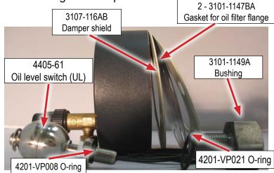
**Step 3.** Reassemble as shown, torque bolts to 72 ft lbs (1000 kg-cm). Leak check, pressurize with nitrogen, then vacuum compressor to 200 microns.
